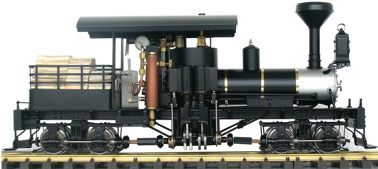
Shay locomotives were developed by Ephraim Shay. His first successful engine that we would recognize today as a Shay locomotive was produced in 1880 by Lima Machine Works (later, Lima Locomotive Works), who would go on to produce approximately 2,700 up until 1945, when production ceased.
